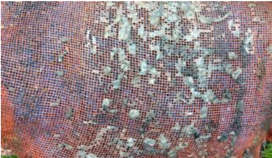
The pictures shows the medias for the growth of the biofilm. It needs not to be removed. Even after a six months holiday period or underload the biological activity will be quickly reactivated and the treatment efficiency will be reached after a short time.
