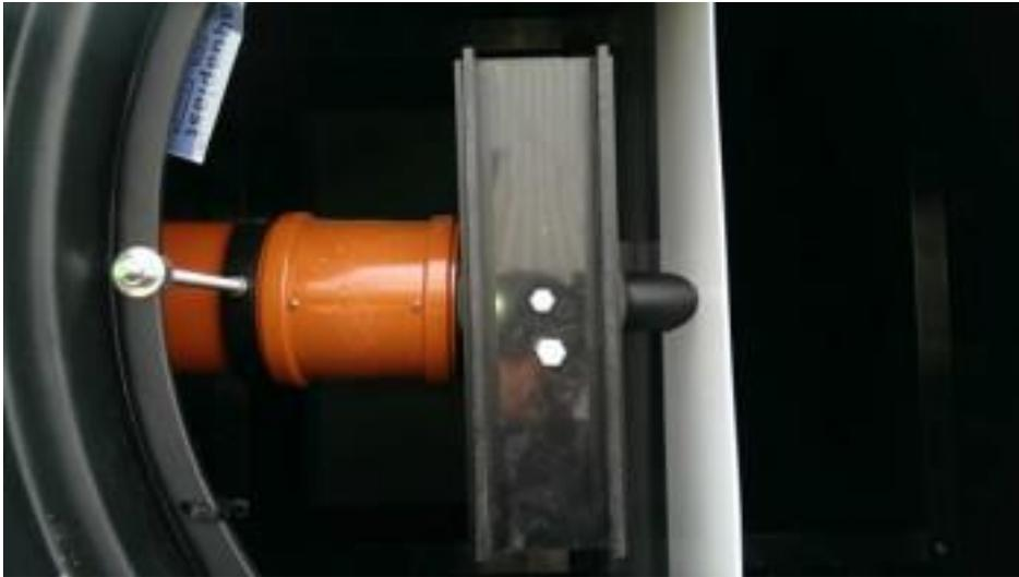
The picture illustrates the function of the ClearFox® nature restriction valve. It equalizes changing inflow and overload. The feed to the biological section will be consistent.
